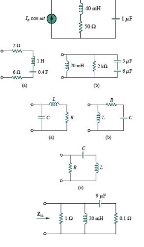
(16) For the circuit shown, find: (a) the resonant frequency  $\omega_o$ (b)  $Z_{in}(\omega)$
